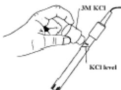
Add in fresh electrolyte until it reaches the level of the refilling port. The reference electrolyte used should be 3M (Mol) KCl. Replace the rubber sleeve.
