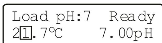
When **Ready** is on the display press **OK** key to start calibration. The message **Wait, please...** appears on the display. Wait for the measured pH value to stabilize. The next message **Load PH 4** will be displayed when the reading is ready. The instrument is calibrated with buffer **pH 7**. To finish the 1-point calibration procedure press button **CAL**.
