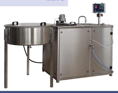
Ekomilk Mini Dairy 120L can be applied for the production of different type of soft and fresh cheese, hard cheese, Yogurt, Pasteurized fresh milk. The installation is designed for processing of up to 120L of milk.
