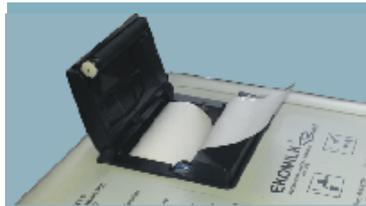
2.3. Loosen the paper end edge from the new paper roll. The end of the paper will be taped or sealed with a sticky material. The paper end edge must be loose. Unroll the loose end 2 to 3 cm from the roll. Place the paper roll in the compartment as is shown on the image.
